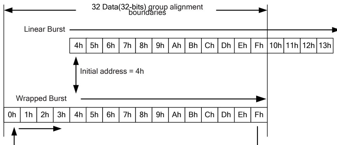
**Figure 4 - Linear Versus Wrapped Burst Sequence**
