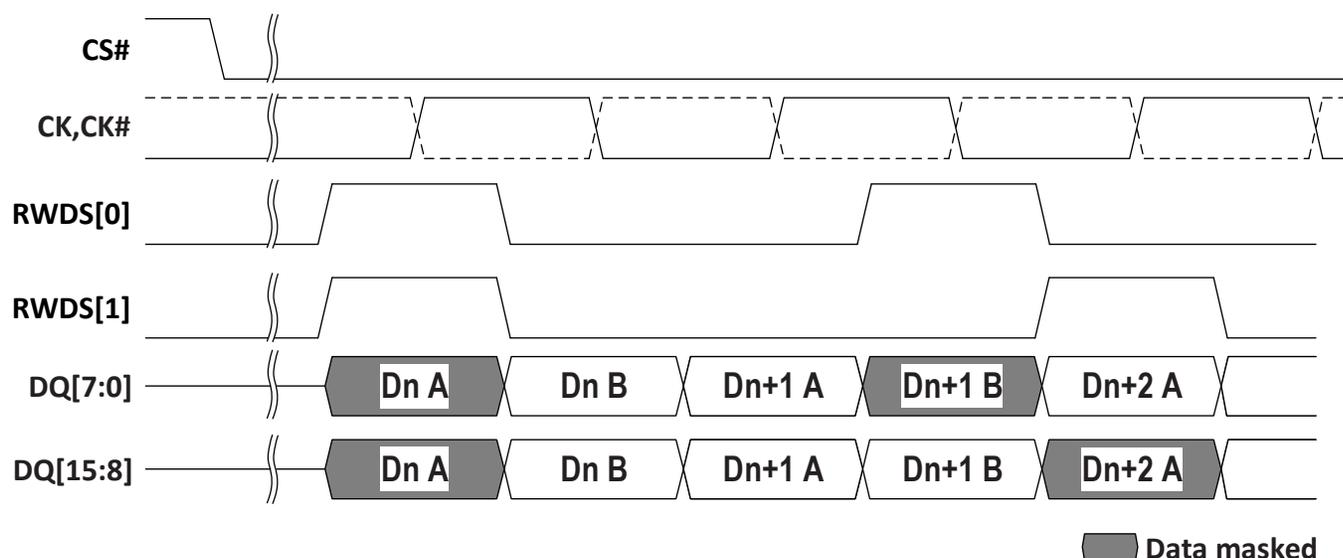
**Figure 7 - Data Placement during a Write Transaction**
