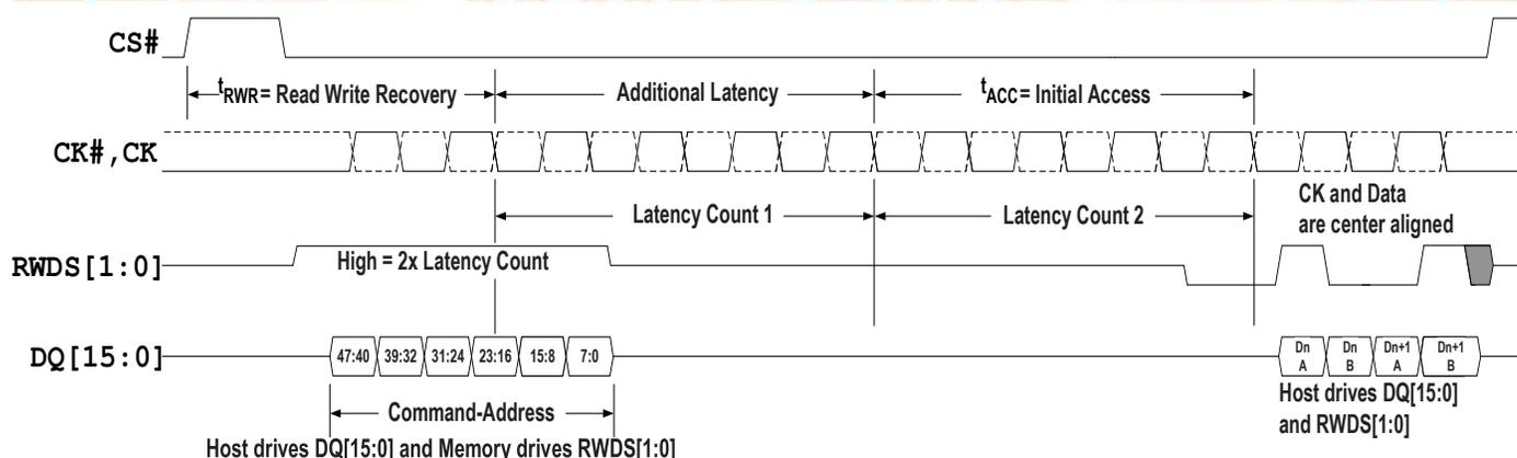
**Figure 10 - Write Transaction with Additional Initial Latency**
