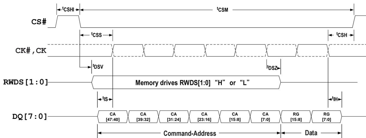
Figure 32 - Write Operation without Initial Latency (Register Write)
