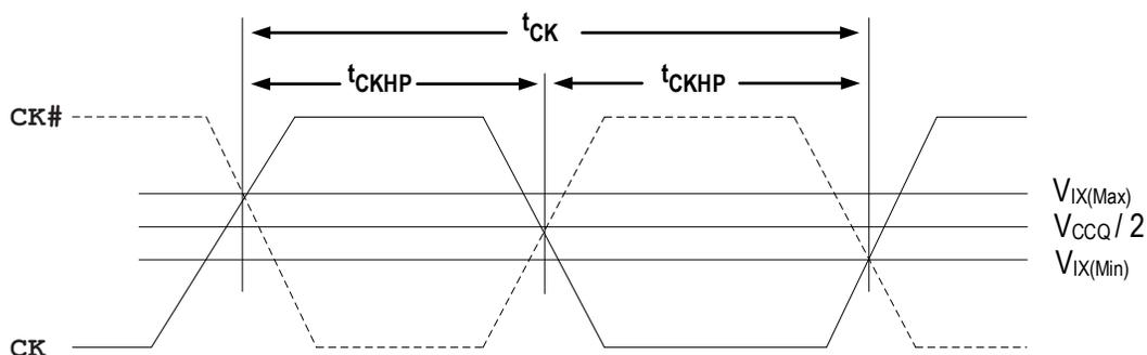
Figure 26 - Clock Characteristics
