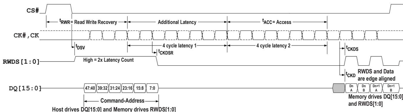
**Figure 28 - Read Timing Diagram — With Additional Latency**
