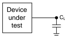
Figure 24 - Test load reference
