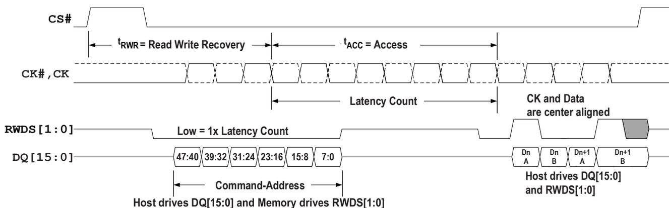
**Figure3 - Write Transaction, Single Initial Latency Count**
