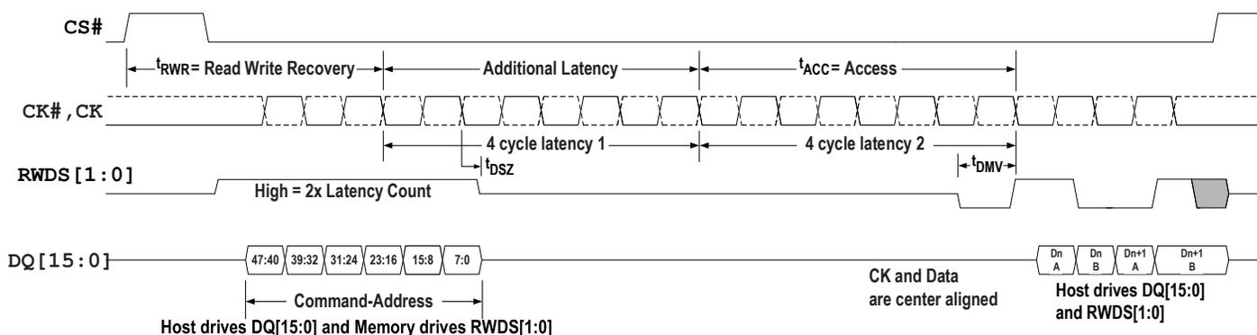
**Figure 31 - Write Timing Diagram — With Additional Latency**
