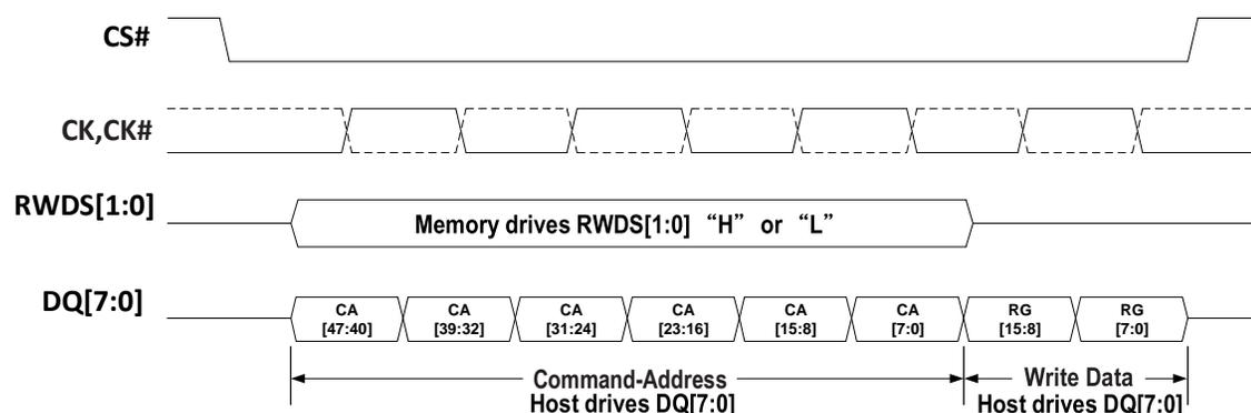
**Figure 12 - Write Operation without Initial Latency (Register Write)**
