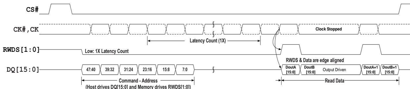
**Figure 13 - Active Clock Stop during Read Transaction (DDR)**
