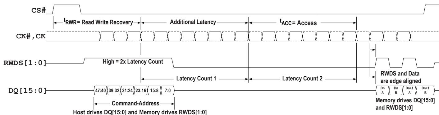
**Figure 8 - Read Transaction with Additional Initial Latency**
