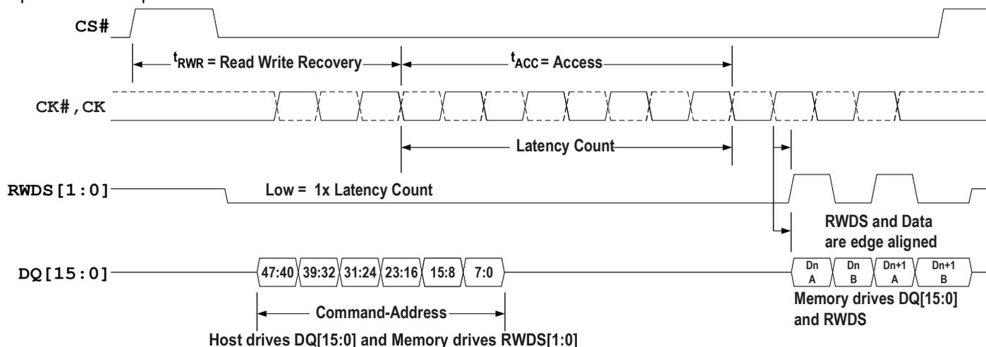
**Figure 1 - Read Transaction, Single Initial Latency Count**
