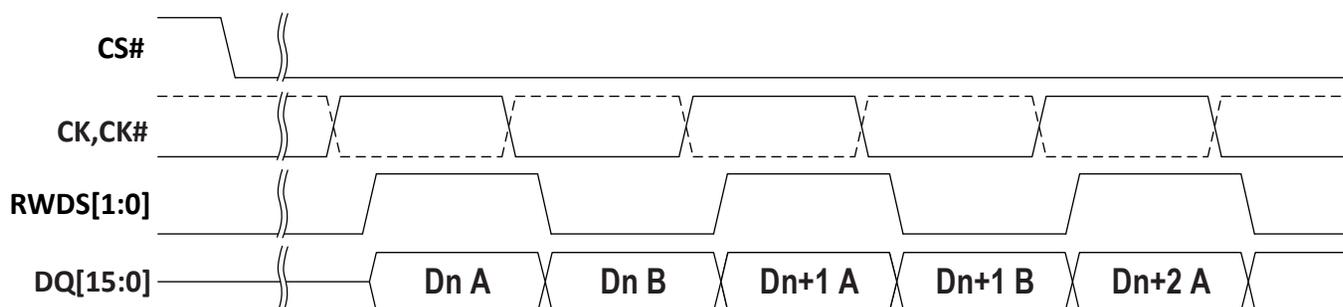
**Figure 6 - Data Placement during a Read Transaction**
